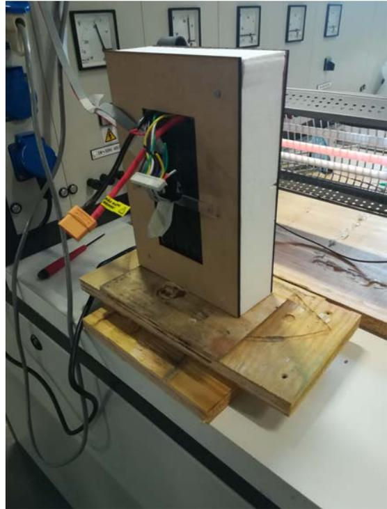
Figure 3.6: Radiation testing for thermal conductivity in the longitudinal direction (6 pouch cells next to each other)
