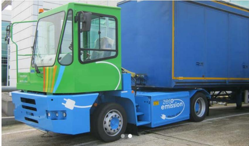
Figure 1.3: Electric terminal truck
