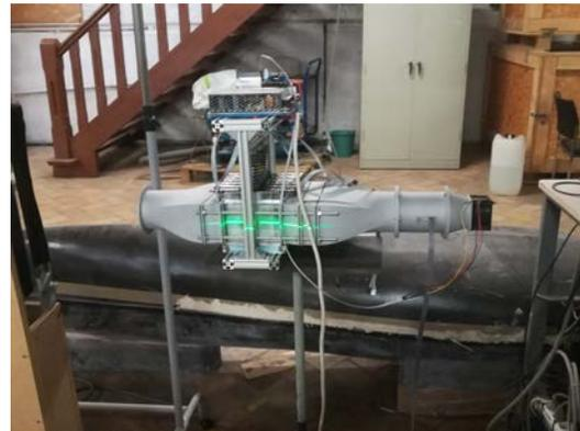
Figure 2.5: PIV measurement synchronised pulsing lazer and camera
